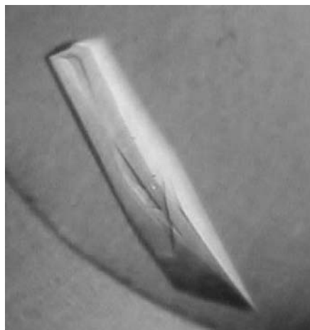
Figure 1 A PEX1 N-terminal domain crystal. The approximate dimensions of the crystal are 0.1 \times 0.1 \times 0.5 mm.
